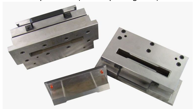
Dismantled punch tool for sheet metal tensile specimens (on tool parking desk)
